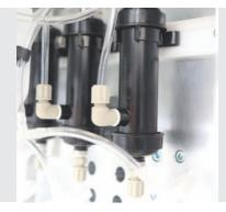
Inline ink degaser. It allows the removal of any I atent air bubble present in the ink, guranteeing the highest print quality.
