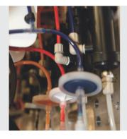
High capacity color tanks (integrated into the machine) allow the high efficiency of the refill process. Inline ink degaser. It allows the removal of any latent air bubbles present in the ink, guaranteeing the highest print quality.
